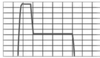
Enhanced spike, for welding very reflective materials with high conductivity (pure copper)
