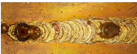
(a) Weld made with traditional fiber laser, 6kW fitted with 100 \mu m fiber, 4mm thick pure copper, 2.5m/min, inconsistent top bead with blow holes and spatter.
