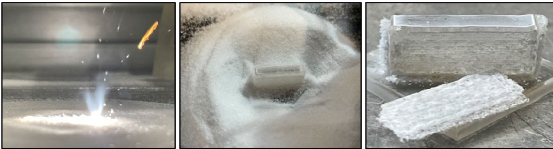
Fig. 6. (a) rim machining after melting; (b) sample in powder bed after building process; (c) edge detachment after manufacturing.
