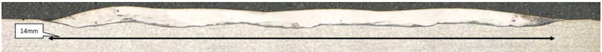
Fig. 10. Four LMD tracks with an oscillation of 1200 Hz (X) and 90 Hz (Y). The robot moved at 8 mm/s and the controller held the temperature at 1800°C.
