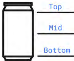
Fig. 3. Diagram of the powder container and heights at which a sample has been extracted.
