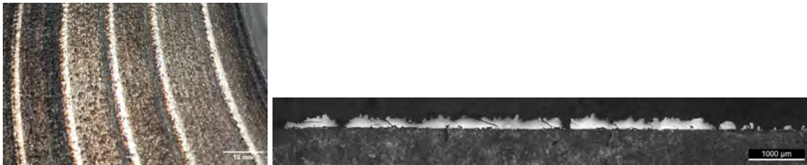
Fig. 12. Surface and cross section images of the cladding deposited with 3 times reused AISI 316L, corresponding Figure 6 (right) PSD.
