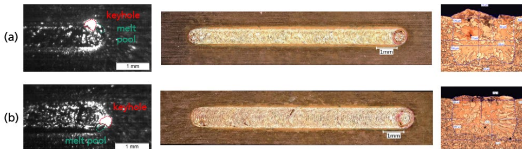
Fig. 7. Possible solutions to avoid humping phenomena during dynamic beam oscillation welding of copper – high speed recording of melt pool, picture of seam surface and cross section for (a) reduction of process interaction zone/amplitude and (b) reduction of beam path speed/frequency
