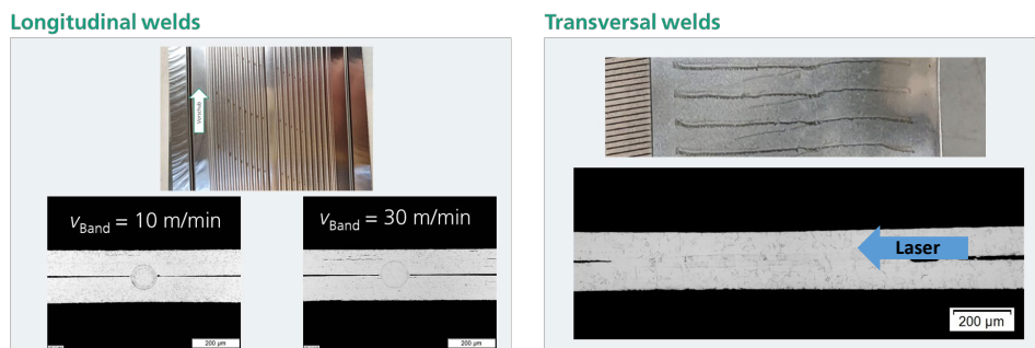
Fig. 5. Longitudinal weld at endless roll-formed strip samples and cross sections at 10 m/min and 30 m/min travel speed (left), transversal welds at flat strip samples and longitudinal cross section (right)
