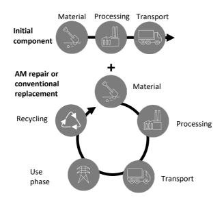
Fig. 2. System boundary of the CO2e assessment: Two stages. 1<sup>st</sup>, upper: Initial component. 2<sup>nd</sup>, lower: Replacement component. The second stage can be either conventional 1-to-1 replacement or AM-repair.
