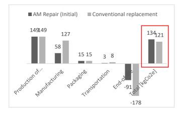
Fig. 3. Initial results of the comparative study of CO<sub>2</sub>e: The conventional replacement emits 13 kgCO<sub>2</sub>e less than the AM-repair.
