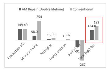
Fig. 6. Assuming the AM-remanufactured component set has double the lifetime of a conventional component set results in app. 48 less kgCO<sub>2</sub>e for the AM remanufacturing.
