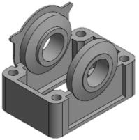
Fig. 1. Simplified CAD-model of the bearing bridge subject to the carbon footprint study (pin bolt not shown).
