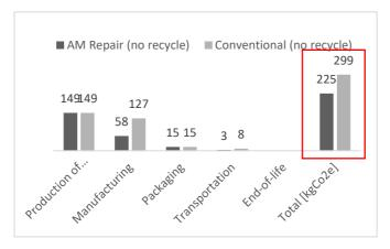
Fig. 4. Assuming no recycling at the end-of-life results in 74 kgCO2e less for the AM remanufactured component set.
