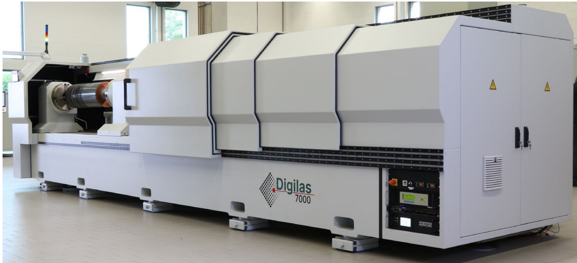
Fig. 1. Cylinder micro processing system, Digilas 7000 for cylinder lengths up to 5m and diameter up to 650mm
