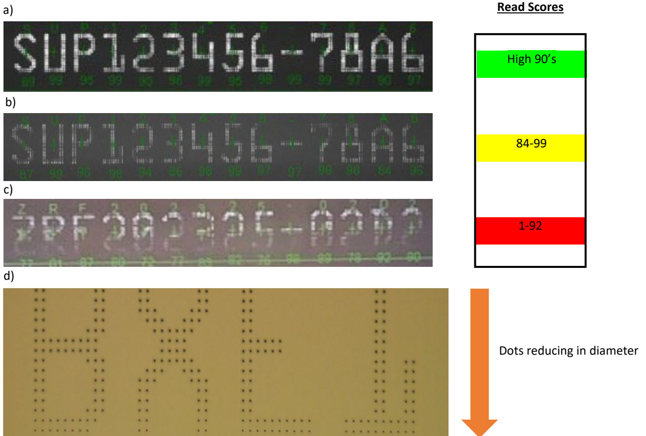
Fig. 1. a) 2W laser running at ~1.5W – Acceptable b) 10W laser running at ~1.5W – Threshold of Acceptable c) 10W laser running at ~1.5W – Failure d) Enlarged image of the 10W laser running at ~1.5W.
