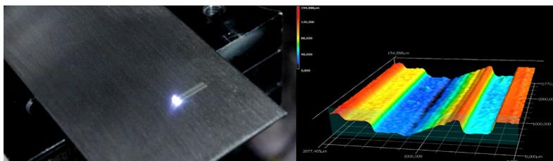
Fig. 6: Generation of groove structure by superimposing beam deflection by galvanometer scanner and AOD. (a) Active machining process; (b) Resulting depth profile of the groove.
