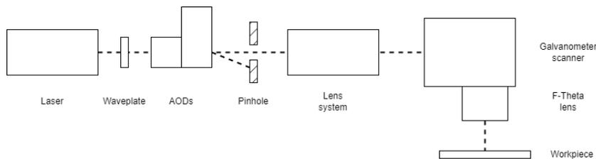
Fig. 3: Schematic representation of the optical setup used for the processes demonstrated in this paper.
