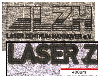
Fig. 4: AODs as a replacement for a galvo scanner. Lasered logo with detail display. Entered bars correspond to 400 µm.
