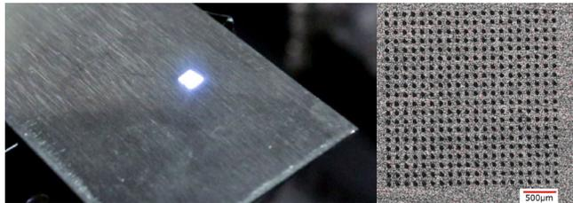
Fig. 5: Generation of a drilling pattern with 400 positions from single pulses using the AOD system. (a) Active machining process; (b) Resulting drilling pattern after 10 laser pulses per hole (10 iterations)
