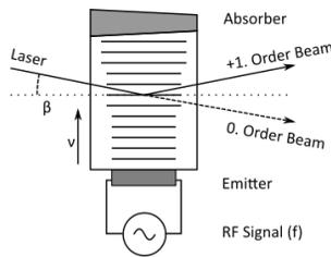
Fig. 1: Structure and function of an acousto-optic deflector.
