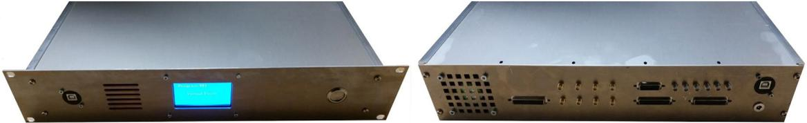
Fig. 2: Front and rear view of the controller for controlling the acousto-optical deflectors.
