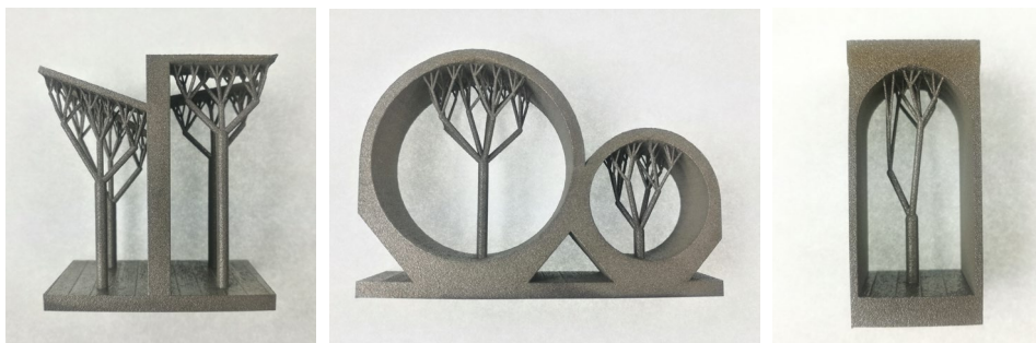
Fig. 7. Printed benchmark parts with BEST supports; (a) Part 1; (b) Part 3; (c) Part 5.
