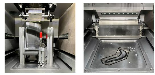
Fig. 3. (a) installation of mounted fixtuing system within SLM 280HL machine; (b) sealed turbine blade leveled during pre processing (root and cooling channels pixelated due to non-disclosure)
