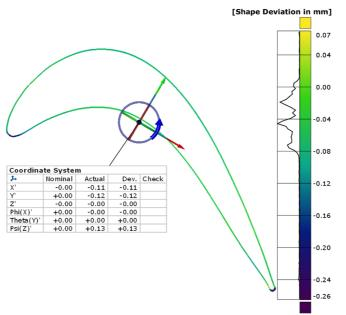
Fig. 4. Evaluation of the shape and position deviation of the hybrid repair process
