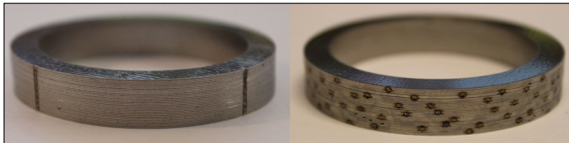
Fig. 1. Different joining strategies of the toroidal cores, Left: Line welds, Right: statistically distributed spot welds
